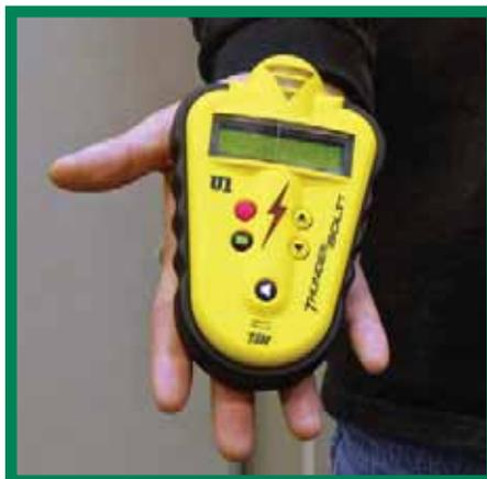
(LEFT) THIS PORTABLE LIGHTNING DETECTOR SOUNDS AN ALARM AND PROVIDES CRITICAL INFORMATION WHEN A LIGHTNING STRIKE OCCURS WITHIN 60 MILES.
