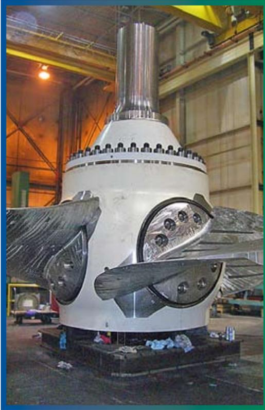
**THE BEEFIER NEW RUNNER HUB IS DESIGNED TO WITHSTAND THE FORCES DELIVERED BY THE ARKANSAS RIVER ONCE IT IS INSTALLED AT OZARK DAM POWERHOUSE.**
